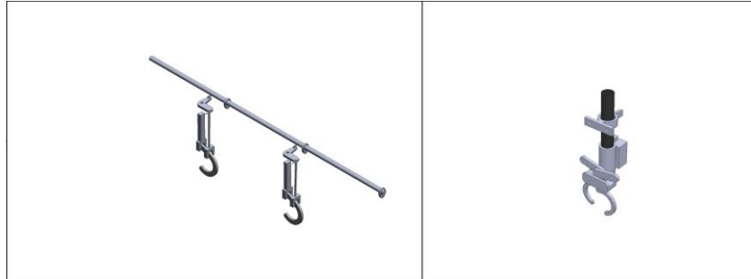
Figure 3.8: Rail Multi Store System and Single Servo Clasp store drop mechanisms
