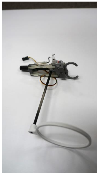
Figure 6.9: Side view of store drop mechanism
