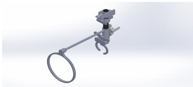
Figure 5.6: Store drop mechanism
