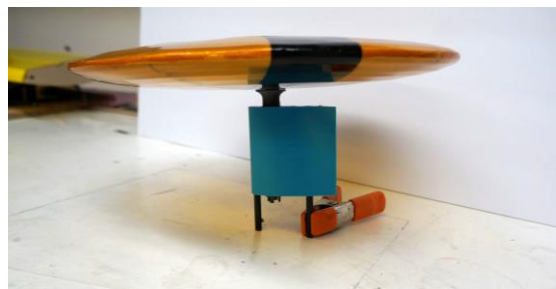
Figure 6.3: Side view of radome with attachment connected
